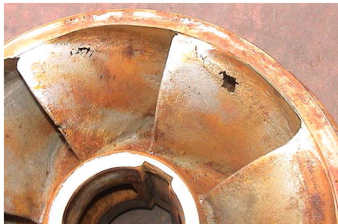
Cavitation suffered Impeller
